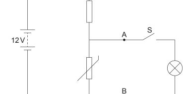
The lamp has a power of 3W at 12V. (i) Use equations from page 2 to calculate the resistance of the lamp at this power and voltage. [3]
